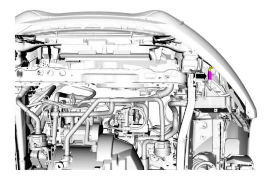
**STEP 7:** Remove 4 push pins and 2 torque screws from lower front bumper cover.
