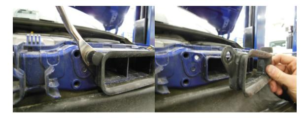
STEP 14: Assemble new air inlet tube by snapping together both pieces. Install onto vehicle through hole in shroud and re-install 2 push pins included in this kit.
