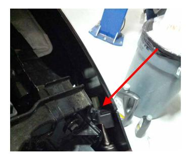
STEP 10: Remove front bumper cover by pulling corners gently out of fenders and by lifting plastic tabs. Carefully set aside on a soft surface to avoid scuffing the paint.
