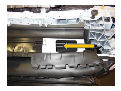
STEP 12: Cut hole in shroud by first drilling a pilot hole. Then, with a proper cutting tool, cut along mark from template.
