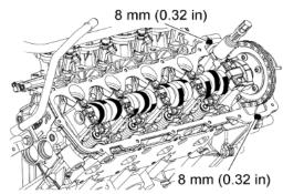
**STEP 2:** Position the RH valve cover and new gasket on the cylinder head and tighten the bolts in the sequence shown below. Tighten the valve cover bolts to 10 Nm (89 lb-in).
