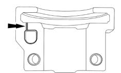
STEP 15: CAUTION: Damage to the camshaft phaser and sprocket assembly will occur if mishandled or used as a lifting or leveraging device.
