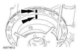
**STEP 4: NOTE:** Do not allow the camshaft roller followers to move out of position when installing the camshaft.
