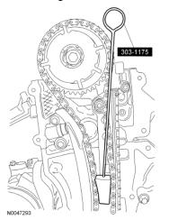
STEP 11: CAUTION: Do not remove the timing chain wedge tool at any time during assembly. If the special tool is removed or out of placement, the engine front cover must be removed and the engine must be re-timed. For additional information, refer to Timing Drive Components in this section.
