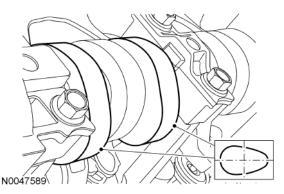
**STEP 9: NOTE:** Do not allow the valve keepers to fall off of the valve or the valve may drop into the cylinder. If a valve drops into a cylinder, the cylinder head must be removed. For additional information, refer to Cylinder Head in this section.
