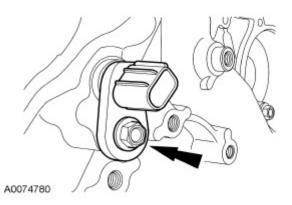
**STEP 11:** Connect the CMP electrical connector.
