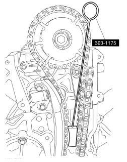
**STEP 7:** Rotate the crankshaft a half turn counterclockwise and position the crankshaft damper spoke at the 12 o'clock position and the timing mark indentation at the 1 o'clock position.
