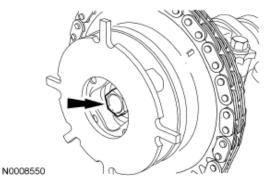
STEP 3: CAUTION: Do not remove the timing chain wedge tool at any time during assembly. If the special tool is removed or out of placement, the engine front cover must be removed and the engine must be re-timed. For additional information, refer to Timing Drive Components in this section.
