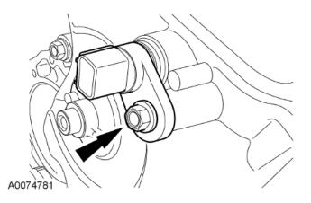
**STEP 11:** Connect the CMP electrical connector.
