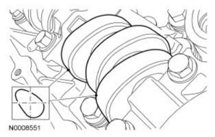
**STEP 9: NOTE:** Do not allow the valve keepers to fall off of the valve or the valve may drop into the cylinder. If a valve drops into a cylinder, the cylinder head must be removed. For additional information, refer to Cylinder Head in this section.
