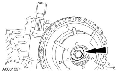
STEP 3: CAUTION: Do not remove the timing chain wedge tool at any time during assembly. If the special tool is removed or out of placement, the engine front cover must be removed and the engine must be re-timed. For additional information, refer to Timing Drive Components in this section.
