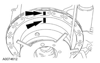
STEP 12: CAUTION: Remove the front thrust camshaft bearing cap straight upward from the bearing towers or the bearing cap may be damaged from side loading.
