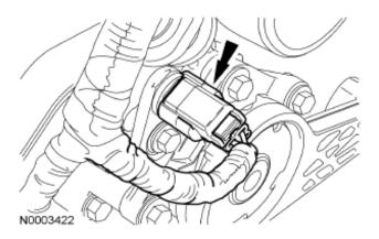
**STEP 5:** Remove the bolt and the RH CMP sensor.
