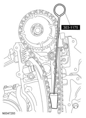
**STEP 7:** Rotate the crankshaft a half turn counterclockwise and position the crankshaft damper spoke at the 12 o'clock position and the timing mark indentation at the 1 o'clock position.
