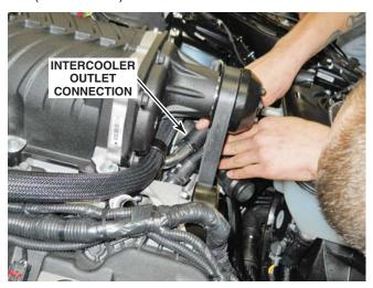
Outlet hose connection at top port of intercooler
