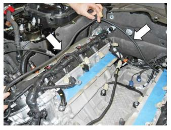
Install the intercooler pump harness red power wire to the first post in the fuse box. Tighten the nut to 10 Nm.
