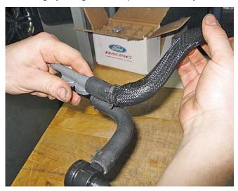
11. Install the hose that goes to the clean air tube (1315-9D691) into the remaining port on the brake aspirator assembly.
