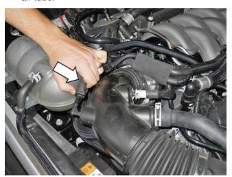
15. Disconnect the vacuum line from the air cleaner tube.
