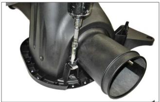
5. Install the Filter (1315-9601R) onto the MAF tube and secure it with the supplied clamp. Torque clamp to 3-5 Nm.
