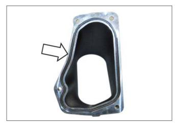
16. Install the Spacer-To-Throttle Body Gasket (R07060153-13) found in Hardware Kit B (1315-TVSHKB) as shown.
