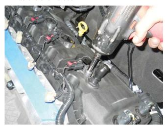
Remove the coil on plug assemblies and label them so they can be reinstalled in their original position. A slight twisting motion will break the seal and ease removal.
