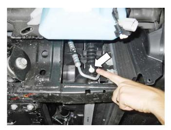
10. If equipped, remove the four (4) nuts and the strut tower cross brace (15 mm socket). The strut tower cross brace cannot be reused after the supercharger has been installed. Discard the nuts.
