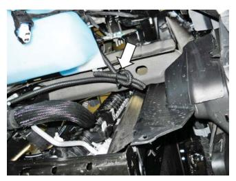
**NOTE:** Route all intercooler hoses very carefully. It is critical for intercooler performance that these hoses are not kinked once installed into the vehicle.
