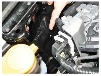
Install the relay and fuse from the Intercooler Pump Wiring Harness (1315-8W501) through the hole and secure it with one (1) M6 x 14 Bolt (N605771) and one (1) M6 Nut (W520412). These parts can be found in Hardware Kit E (1315-TVSHKE).
