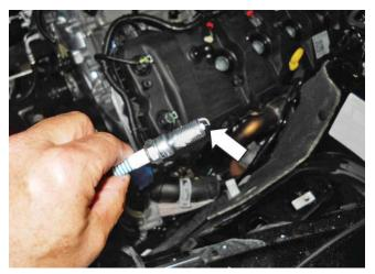
7. Install the new spark plugs using a 5/8" spark plug socket and 6" extension. Torque to 14 Nm.
