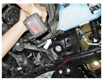
3. Install the Intercooler Pump (F8YH-8501) into the Pump Retainer (R07070065-4G) and onto the intercooler pump bracket. Secure the pump and retainer to the bracket using one (1) M6 x 16 Bolt (N605891). Torque the bolt to 10 Nm.
