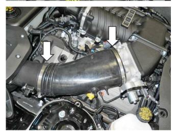
6. Install the PCV Fresh Air Inlet Tube (1315-6758) by connecting the 90-degree fitting to the driver side cam cover and angled fitting to the PCV fitting in the clean air tube.
