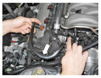
25. Disconnect the fuel supply hose from the fuel rail. **NOTE:** Use a rag to catch any excess fuel during disconnection. Use a cap, tape or other suitable method to block the rail opening from contaminants.
