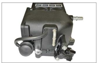
4. Connect the brake boost hose to the 90-degree tube at the rear of the supercharger and secure it with the clamp. This is "hose 1" created from the brake boost vacuum and aspirator assembly modification process.
