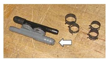
8. Use the takeoff clamps and attach them to the aspirator to brake booster hose (1315-9D690).
