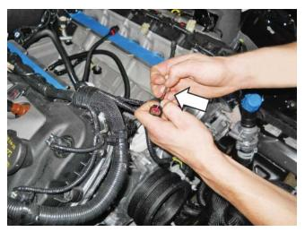
2. Depress the locking tab and separate the "empty" female 1 x 2 connector from the Evaporative Emissions Canister Purge Valve Extension Harness (13119G866). This connector replaces the connector removed in the previous step. Carefully pull the white locking tab forward to allow wires to be installed into the connector. Populate the new connector such that the white with brown wire is in position 1 and the green wire is in position 2. Depress the white locking tab to secure the wires.
