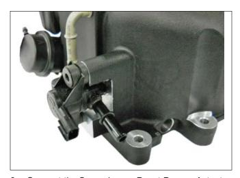
Connect the Supercharger Boost Bypass Actuator Hose (1315-9E498) found in Hardware Kit D (1315-TVSHKD) to the top port on the actuator and route to the small port on the supercharger.
