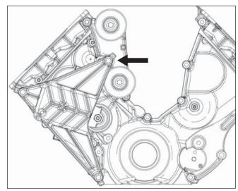
11. Using a 17 mm socket, rotate the new tensioner clockwise to install the belt on to the supercharger pulley. Inspect each pulley to ensure the belt is properly seated. Ensure all supercharger pulley bolts have been torqued to 10 Nm.
