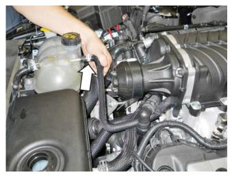
8. Ensure that all intercooler hoses, the degas hose and all clamps and wiring have been installed to provide maximum clearance to the supercharger belt.
