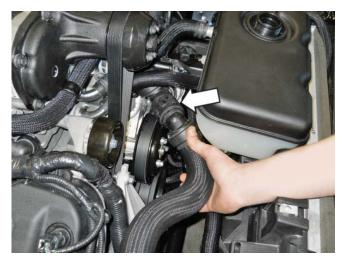
2. Reconnect the other end of the coolant hose to the upper RH inlet of the radiator. Secure it with the clamp.
