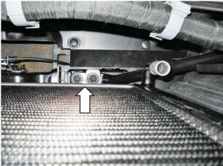
4. Install two (2) J-Clips (W520823) on both frame rail ends as shown. Some trimming of the J-Clip may be required to install the J-Clip through the hole in the frame.
