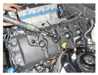
8. Apply a small amount of dielectric grease to the inside of the coil on plug boots before attaching to the spark plugs. Install the ignition coil on plugs in their original position. Install the coil on plug bolts and torque to 6 Nm.
