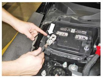
5. Release the (8) push pin retainers by pulling the center pin and remove the radiator trim cover.
