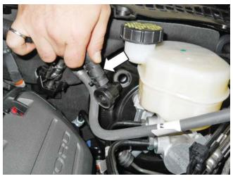
30. Remove the brake boost vacuum hose/line from the vehicle and set it aside. This line will be modified.
