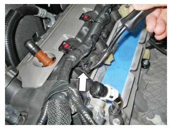
Peel back the insulation at the base of the ground wire that was attached to the stud on the front cover. Trim back part of the insulation until the ground wire is exposed.
