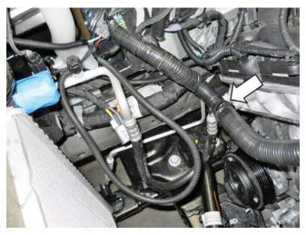
9. Route the intercooler pump wire harness over the top and in front of the wiper washer bottle. Secure it in place with zip ties as necessary.
