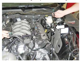
24. Remove the PCV Purge line from the intake manifold and RH cam cover. This line will not be reused.
