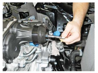
12. Install the brake aspirator hose assembly.
