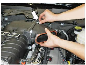
18. Connect the fuel supply line to the fuel rail and lock it into position.
