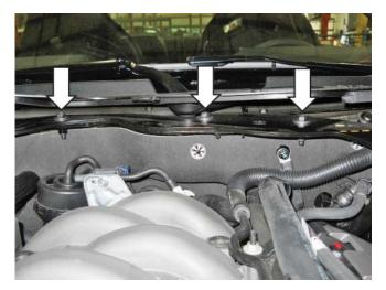
13. Pry up the pushpin securing the induction resonance tube to the strut tower. Remove the mounting nut at the base of the induction resonance tube at the firewall (10 mm). If necessary, remove the dipstick to gain access to the nut. Remove the induction resonance tube from the cowl. The induction resonance tube will not be reused.
