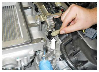
Carefully place the Supercharger Assembly (1315-6F066) on top of the intake manifold. Ensure that the supercharger is fully seated on the intake mounting dowels. Remove protective shipping covers.
