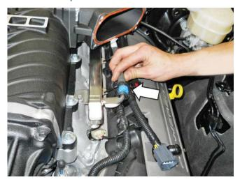
Install the Throttle Body Assembly (R07060150) on the throttle body spacer. Use four (4) M6 x 32.5 mm Bolts (R18020009) found in Hardware Kit B (1315-TVSHKB) to secure the throttle body assembly to the spacer. Torque bolts to 10 Nm.
