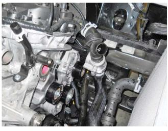
54. Remove the four (4) water pump mounting bolts (10 mm socket) and remove the water pump. Set both aside for re-use.
