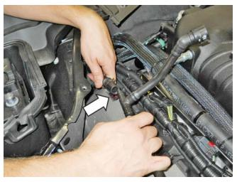
32. Connect the PCV Purge Line (13116K817) to the PCV Valve on the RH cam cover and the port on the RH side of the supercharger.
