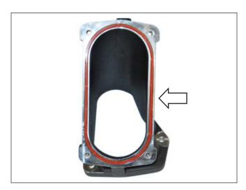
17. Mount the Throttle Body Spacer (1315-9P697) using four (4) M6 x 32.5 Fasteners (R18020009). These parts can be found in Hardware Kit B (1315-TVSHKB). Torque the fasteners to 10 Nm.
