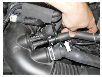
17. Disconnect the PCV Fresh Air Inlet tube from the left-hand cam cover and remove the tube from the vehicle.
