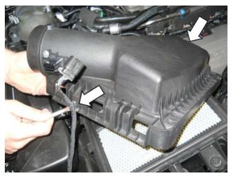
20. Remove the filter from the airbox. Remove the mounting bolt at the side of the airbox (10 mm socket). Pull up and remove the lower airbox from the vehicle.
