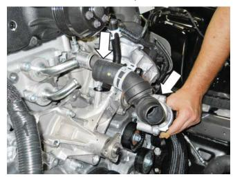
5. Install the two (2) thermostat housing mounting bolts and torque to 10 Nm.
