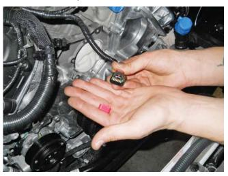
3. Populate the new connector such that the yellow with violet wire is in position 1, the blue with green wire is in position 2, the brown wire is in position 3, the blue with orange wire is in position 4, the yellow wire is in position 5 and the green with violet wire is in position 6. Install the red plastic lock into the connector to secure the wires in place.
