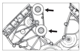
8. Route the FEAD Belt (K060806) as shown. Do not route the belt onto the supercharger pulley.
