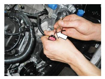
2. Depress the locking tab and separate the "empty" female 1 x 6 connector from the new TPS/ETC Extension Harness (131114A595). It will be used in the next step.
