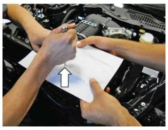
2. Use a dremel or other suitable tool to remove material in the three (3) rectangular areas marked as well as the two (2) holes.
