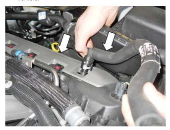
18. Loosen the clamps securing the clean air tube at the airbox and throttle body. Remove the clean air tube from the throttle body and airbox lid. The clean air tube will not be reused.
