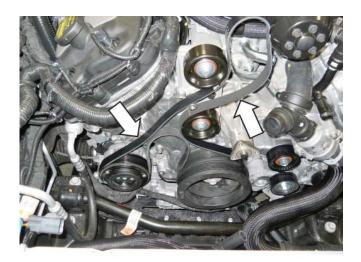
Loosely install the FEAD Tensioner Bracket Assembly (13118B603) onto the front cover using two (2) M8 x 1.25 x 120 mm Bolts (N811329) found in Hardware Kit C (1315-TVSHKC).
