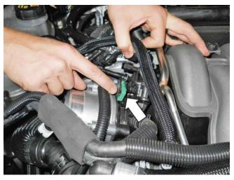
**EECPV** tube quick connector with green lock
