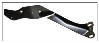
3. Use a suitable tool to file the sharp end where the brace was cut.
