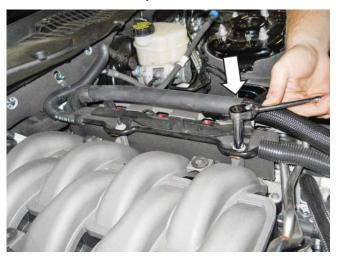
29. Disconnect the brake boost vacuum hose from the port at the firewall.
