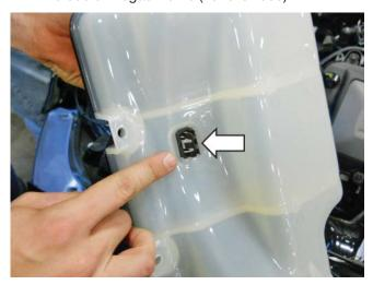
Position the intercooler degas bottle to the fan shroud and check the fit, but do not install.
