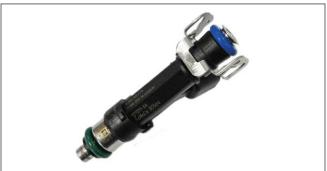
2. Apply assembly lube to the injector O-rings and install the injectors into the new Fuel Rail (1315-19F792).
