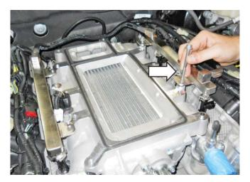
8. Connect the eight (8) fuel injector electrical connectors.
