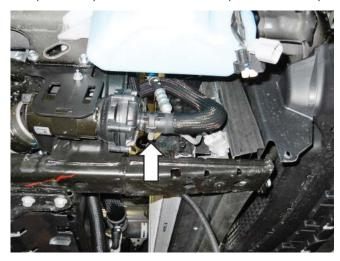
Install the Intercooler Degas Bottle Inlet Hose (1315-8D031) to the outlet on the intercooler.
