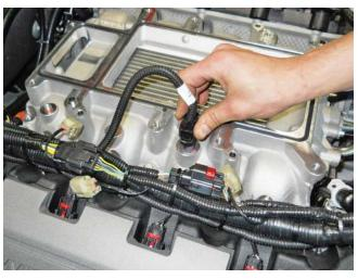
7. Lube the lower fuel injector O-rings with assembly lube. Install the fuel rail and injectors into the intake manifold. Be sure each injector is properly seated into the intake manifold. Install the previously removed fuel rail mounting bolts. Tighten the fasteners in two stages with the sequence shown. Stage 1; torque bolts to 10 Nm. Stage 2; tighten bolts an additional 45 degrees.
