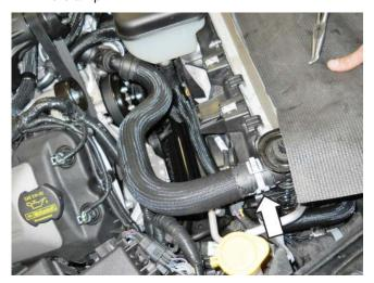
3. Reinstall the factory degas bottle onto the fan shroud and torque the bolts to 10 Nm.
