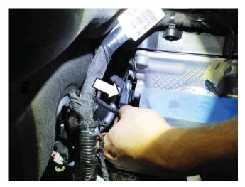
4. Route the intercooler pump wire harness in back of the cylinder head along the RH engine harness to the area near the fuse box.
