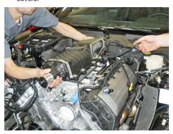
Install the ten (10) M8 x 1.25 x 53 Fasteners (N808130) provided found in Hardware Kit B (1315-TVSHKB) into the mounting holes. Torque fasteners to 25 Nm in the sequence shown (10 mm socket).
