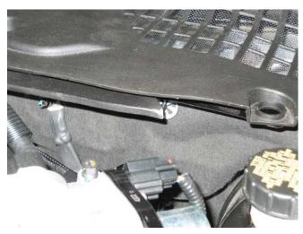
Exposed point on modified K-brace, shown installed
