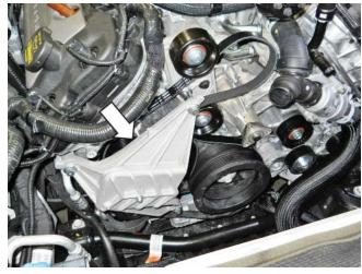
Install one (1) M8 x 1.25 x 41 mm Bolt (W705128) found in Hardware Kit C (1315-TVSHKC), to fasten the Tensioner Bracket to the Upper FEAD Bracket. Torque all three (3) Tensioner Bracket bolts to 25 Nm.
