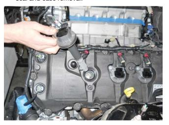
Use a 5/8" spark plug socket and 6" extension to remove the eight (8) factory spark plugs and set aside. These will not be re-used.
