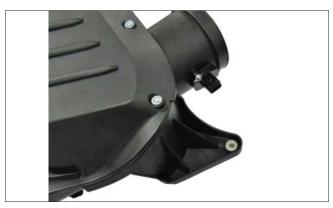
10. Remove the rubber mounting isolator from the bottom of the factory airbox and install it onto the mount on the bottom of the new airbox in the same orientation.
