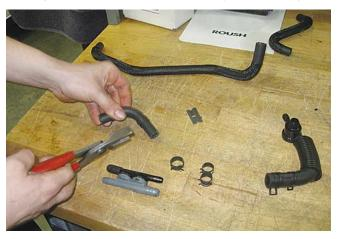
Install the aspirator to brake booster line (1315-9D690) into the black port on the brake aspirator assembly. Then install the check valve that plugs into the brake booster.
