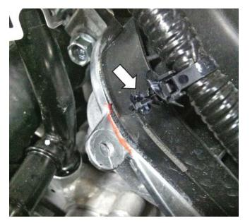
4. Remove the wiring retention clip from the feature on the front cover and set aside.
