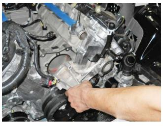
55. Place a clean towel in the water pump inlet cavity.
