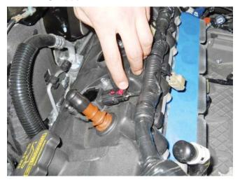
10. Re-install the coil on plug covers. Reinstall the oil cap after the RH cover is installed.
