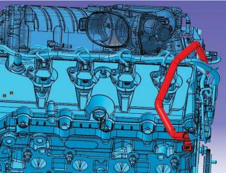
23. Connect the new Evaporative Emission Canister Purge Valve Line (1315-9G271), to the relocated Evaporative Emission Canister Purge Valve on the back of the supercharger. Slide the green clip to lock the connector. **Make sure the hose is routed away from any hot surfaces.**
