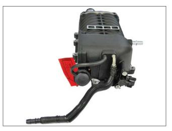
5. Connect the Supercharger Bypass Reference Vacuum Line (7R3V-9E498) to the bottom fitting on the supercharger bypass actuator.
