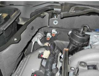
34. Disconnect the clamps on the hose ends and remove the 3/8" engine coolant degas hose from both the engine and the degas bottle.
