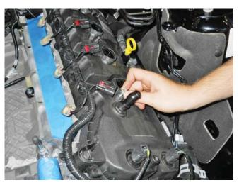
9. Connect the electrical connectors for each ignition coil eight (8) places.
