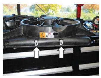
Insert the Clip (20860) found in Hardware Kit H (1315-TVSHKH) onto the tab on the bottom of the Intercooler Degas Bottle (1315-8D080).
