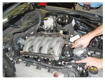
41. Clean the intake mounting surfaces and apply tape over the open intake ports to prevent engine contamination.
