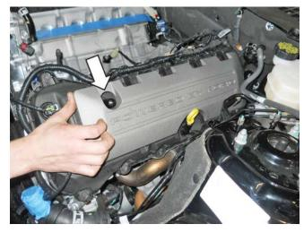
Disconnect the electrical connectors for each ignition coil (eight [8] places).
