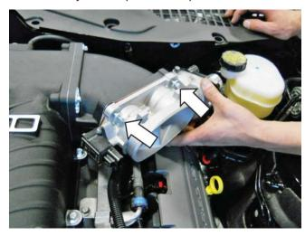
20. Install the ETC and TPS electrical connectors to the throttle body.
