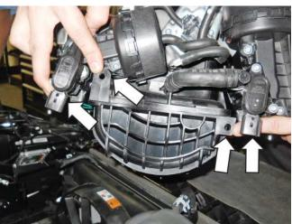
Harness push pin retainer points on rear of intake
