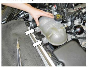
4. Install the engine degas bottle hose on the rear of the bottle and to the upper LH radiator. Secure both ends of the hose with the clamps.
