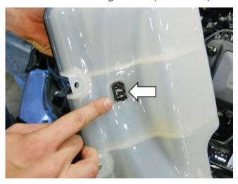
Install the Intercooler Pump Inlet Hose (1315-8D029) to the bottom of the intercooler degas bottle and secure it with the Clamp (CT19X12).
