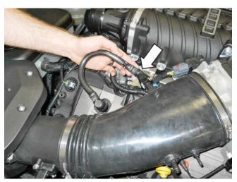
Route the MAF wire harness around the airbox assembly and connect the harness to the MAF sensor. Make sure the red lock is engaged on the connector.
