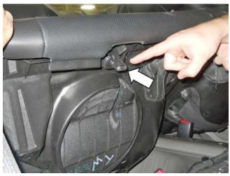
b. Disconnect the Fuel Pump Control Module electrical connector located under the driver side back seat.
