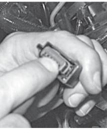
4. Connect the TPS/ETC Extension Harness (131114A595) from Hardware Kit E (1315-TVSHKE) to the newly installed connector. The wire colors on each side of the connector pair should align. Route the harness along the main wiring harness to the rear of the driver side cam cover. Use tape or zip ties to secure the extension harness to the main harness.
