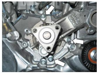
4. Install the thermostat housing and hose assembly and secure it with the clamp.
