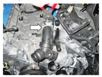
52. Remove the two (2) bolts from the thermostat housing (8 mm socket).
