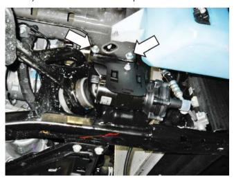
Install the intercooler pump outlet hose (1315-8K236) from the pump outlet, over the side of the frame rail and to the inlet on the lower RH side of LTR.
