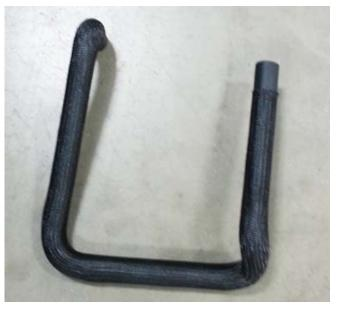
Intercooler pump outlet hose (1315-6K236)
