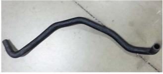
Intercooler pump inlet hose (1315-8D029)
