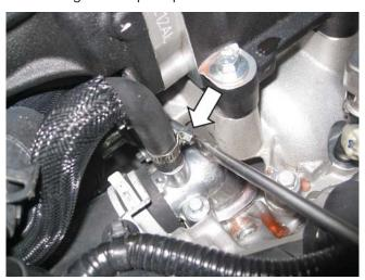
Install the other end of the hose to the engine degas bottle as shown. Secure the constant tension clamp.
