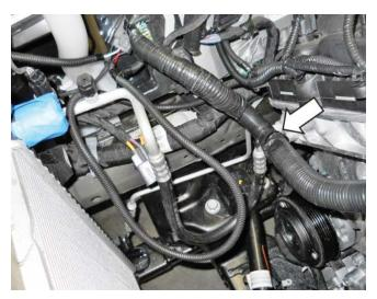
10. Route the intercooler pump wire harness over the top and in front of the wiper washer bottle. Secure it in place with zip ties as necessary.
