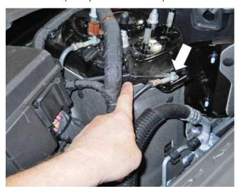
8. Route and tuck the intercooler pump harness under the engine harness and down the RH coil cover towards the fuse box as shown. Secure it in place with zip ties.
