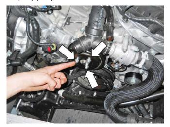
49. Cut and remove the A/C compressor belt. Discard belt.
