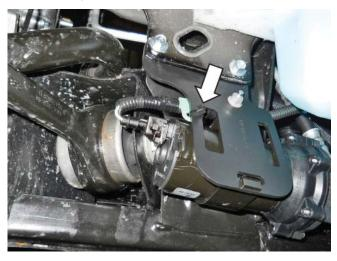
8. Collect the excess intercooler pump harness and secure it with zip ties as needed.
