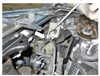
2. Install the Dirty Air Duct (1315-9F763) at the LH side of the radiator.
