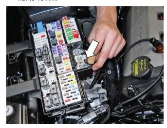
6. Install the ground wire with the existing ground wire near the RH strut tower and retighten the bolt to 10 Nm. Coil up the extra wire slack.
