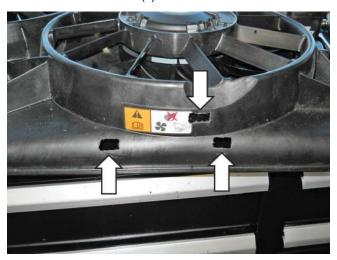
3. Install two (2) J-Clips (N623332-M6) found in Hardware Kit H (1315-TVSHKH) in the two (2) areas on the edge of the shroud.
