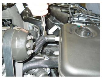
Install the hose to the intercooler cooler outlet using (1) Clamp (CT19X12) from Hardware Kit G (1315-TVSHKG).
