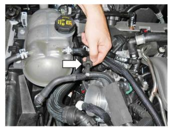
22. Disconnect the throttle body electrical connector. Pull the red locking tab back; press the black release tab to disengage the lock.
