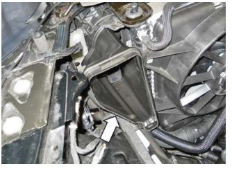
Lower the airbox assembly into mounting position. Align the airbox assembly opening with the dirty air duct and press it into the dirty air tube until properly installed. A snap will be heard when properly seated.
