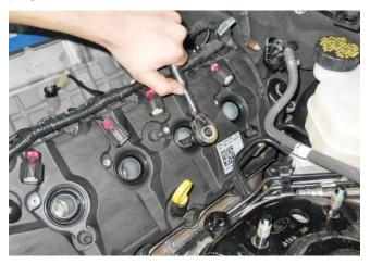
Unpack the eight (8) provided Spark Plugs (BL3E-12405) which are pre-gapped to 0.9 mm. Check to ensure the gap is intact and none are damaged.
