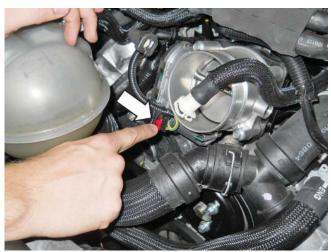
23. Unlock the green connector and disconnect the evaporative emission canister purge valve (EECPV) tube and electrical connector (green). Remove the EECPV tube retainer from the front left hand cam cover. Disconnect the remainder of the tube at the fitting located behind the inner fender (pry from retainer) below the brake booster. Remove from vehicle and set it aside. The quick connect (green locking) connectors must be transferred to the new line in Hardware Kit E.
