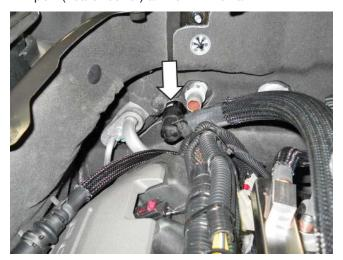
28. Install the 424mm length of protective hose sleeve (1311-18K579) found in hardware kit D (1315-TVSHKD) over the RH factory heater hose and secure with tape on either end of the sleeve. Reinstall the RH factory heater hose to the tube at the RH front of the engine.
