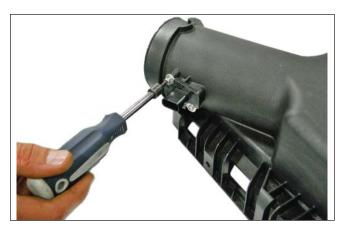
7. Transfer and install the factory MAF sensor into the MAF tube assembly using the original MAF sensor bolts (M4 X 0.7 X 10) and tighten with a T-20 Torx bit. Torque the screws to 1.8–2.2 Nm. Be careful not to over tighten these screws. Wiggle the MAF sensor to ensure that it is properly fastened.
