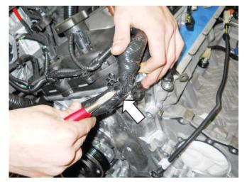
2. Route both extension harnesses along the engine harness. Secure them in place with zip ties.
