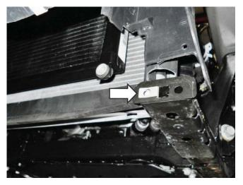
5. Install the RH LTR Support Bracket (1315-8K245) and LH LTR Support Bracket (1315-8K244) found in Hardware Kit H (1315-TVSHKH) on the lower tabs. Make sure to install the LH and RH in the correct position with the correct orientation. Secure each bracket at the radiator using a Bolt (W705128) and Nut (W520413). Secure each bracket to the chassis using a Bolt (W705128) through the J-Clip. Torque to 25 Nm.
