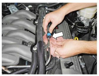
26. Disconnect the brake booster vacuum hose from the intake manifold. This port is located directly behind the throttle body.
