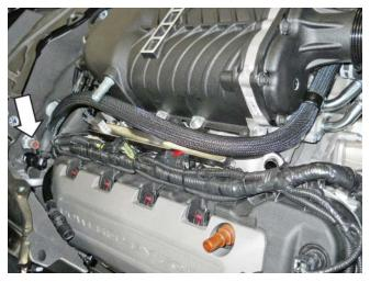
27. Install the heater hose connector to the bottom port (heater outlet) at the RH firewall.
