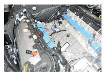
4. Wrap electrical tape around the two (2) blue CMCV connectors at the rear of the cylinder head as shown.
