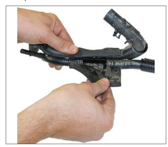
6. Release the clamp and separate Section B, hose 2, from the steel tube. Disassemble the remaining brake aspirator assembly. Keep all clamps since they will be reused.
