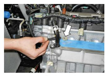
Use snips to cut off the bent metal tab on the end of the ground tab.
