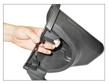
3. Place the MAF Tube Assembly (1315-12B579HC) through the opening of the airbox tray from the inside.
