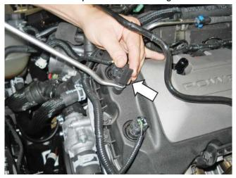
Remove retainer on cam cover
