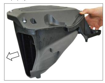
4. Secure the airbox using the M6 bolt from the original airbox and torque to 10 Nm.
