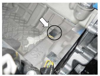
Use a grinder or suitable tool to grind the boss down across the entire length. Make sure to take off material uniformly along the angle. If high spots are left, the intake manifold will not seat properly on the engine.
