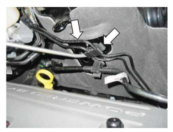
Remove tube from retainer
