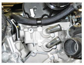
26. Route the hose along the RH fuel rail and down to the heater outlet at the firewall.
