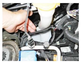
10. Zip tie the excess harness out of the way and secure it to a safe location.
