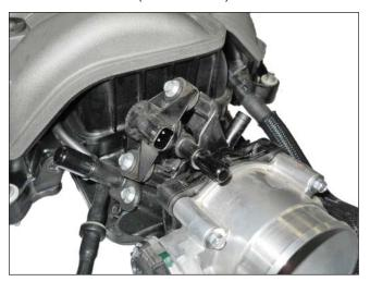
Install the valve into the rear of the supercharger (1315-6F066) using two (2) M6 x 1.0 x 35.5mm Bolts (N808429) found in Hardware Kit B (1315-TVSHKB). Torque bolts to 8-12 Nm.
