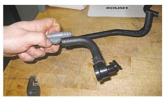
10. Install the line that goes from the supercharger to the aspirator assembly (1315-9D692) into the 1/2-inch grey fitting on the aspirator assembly.
