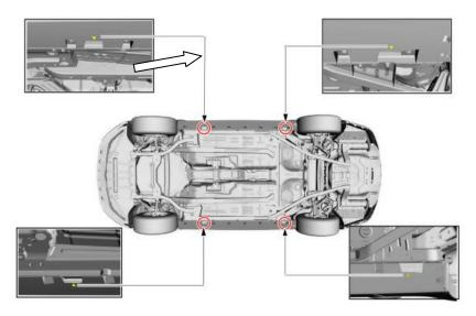
**STEP 2:** Locate the (4) existing holes in the front engine cradle.
