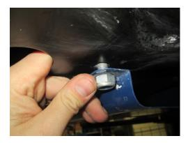
STEP 7: Tighten the (2) rearward M10 x 60mm bolts and torque to 31 ft lbs.
