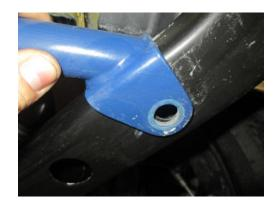
**STEP 4:** Position the (2) provided sleeves over the (2) provided M10 x 60mm bolts.
