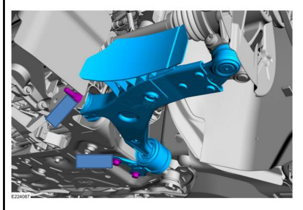
Slide deflectors onto the lower control arm. Install push pins to retain the deflector.
