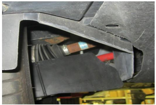
Trim inner wheel wells to allow direct air flow to deflectors. (RH side show)
