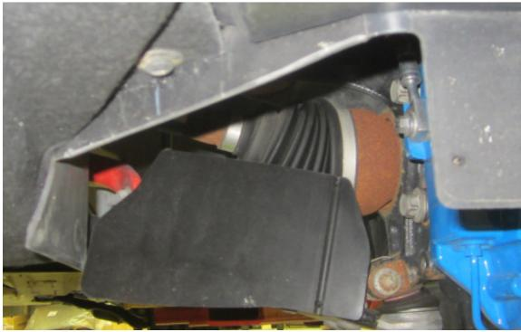
Trim inner wheel wells to allow direct air flow to deflectors. (LH side shown)
