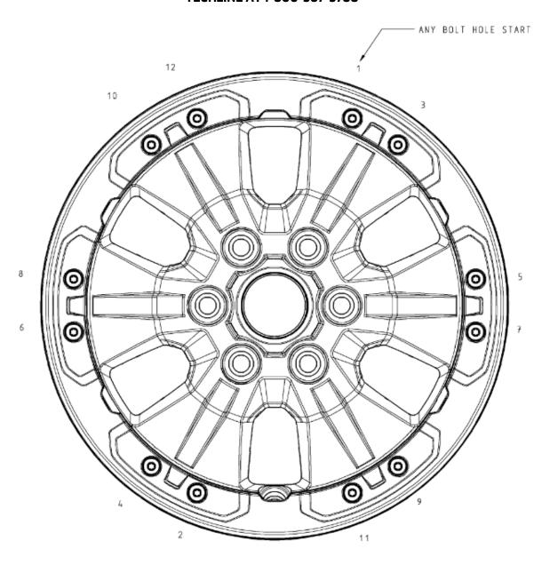
Step 1. Hand tighten all bolts in sequence. Step 2. Final torque in sequence 17.5 N.m.
